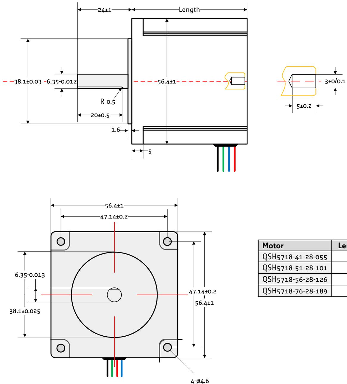
Figure 4.1: Dimensions of QSH5718. All values in mm.
