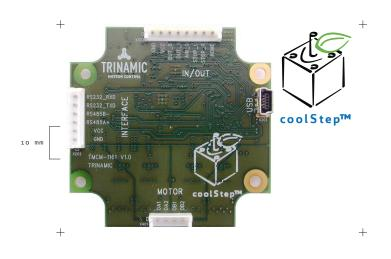
INFO The TMCM-1161 is an intelligent stepper motor controller/driver module featuring the new outstanding coolStep<sup>™</sup>
