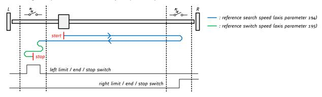
Figure 4.4: Search right stop switch, then search left stop switch from both sides
