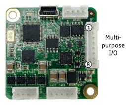
Figure 3.2 I/O connector
