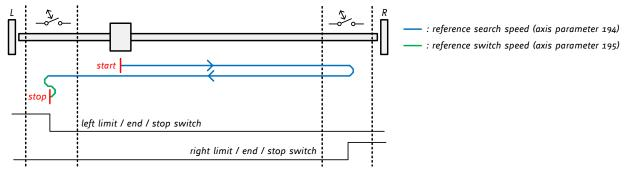
Figure 4.3: Search right stop switch, then search left stop switch
