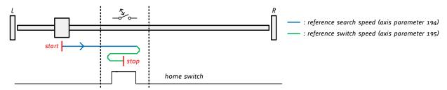
Figure 4.9: Search home switch in positive direction, ignore end switches
