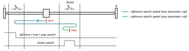
Figure 4.6: Search home switch in negative direction, reverse direction in case left stop switch is hit
