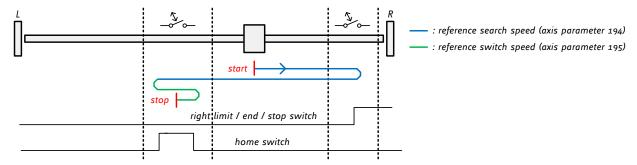
Figure 4.7: Search home switch in positive direction, reverse direction in case right stop switch is hit
