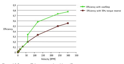
Figure 1.2 Energy efficiency example with coolStep
