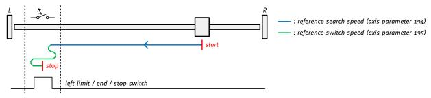
Figure 4.5: Search left stop switch from both sides
