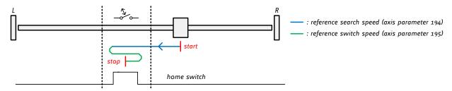
Figure 4.8: Search home switch in negative direction, ignore end switches
