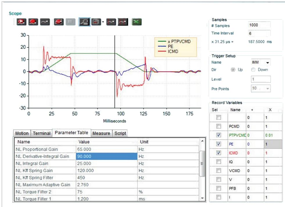
**Figure 12-31. NLPEAFF 120 Hz - Minimum position error, but some oscillations at stop**
