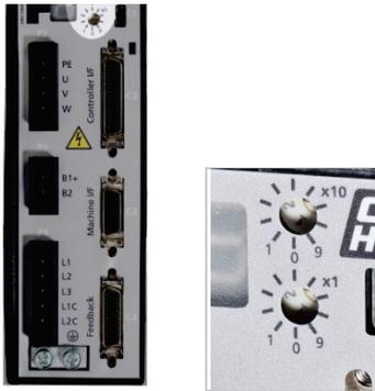
Figure 3-12. Drive Address Rotary Switches
