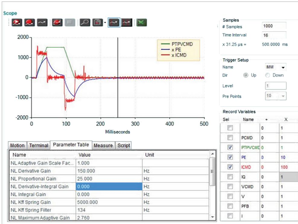
Figure 12-14.KNLP 25 Hz – Position error reduced
