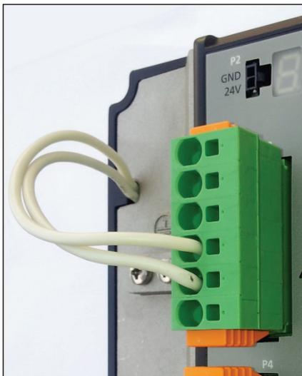
**Figure 3-23. External Regeneration Resistor Wiring**
