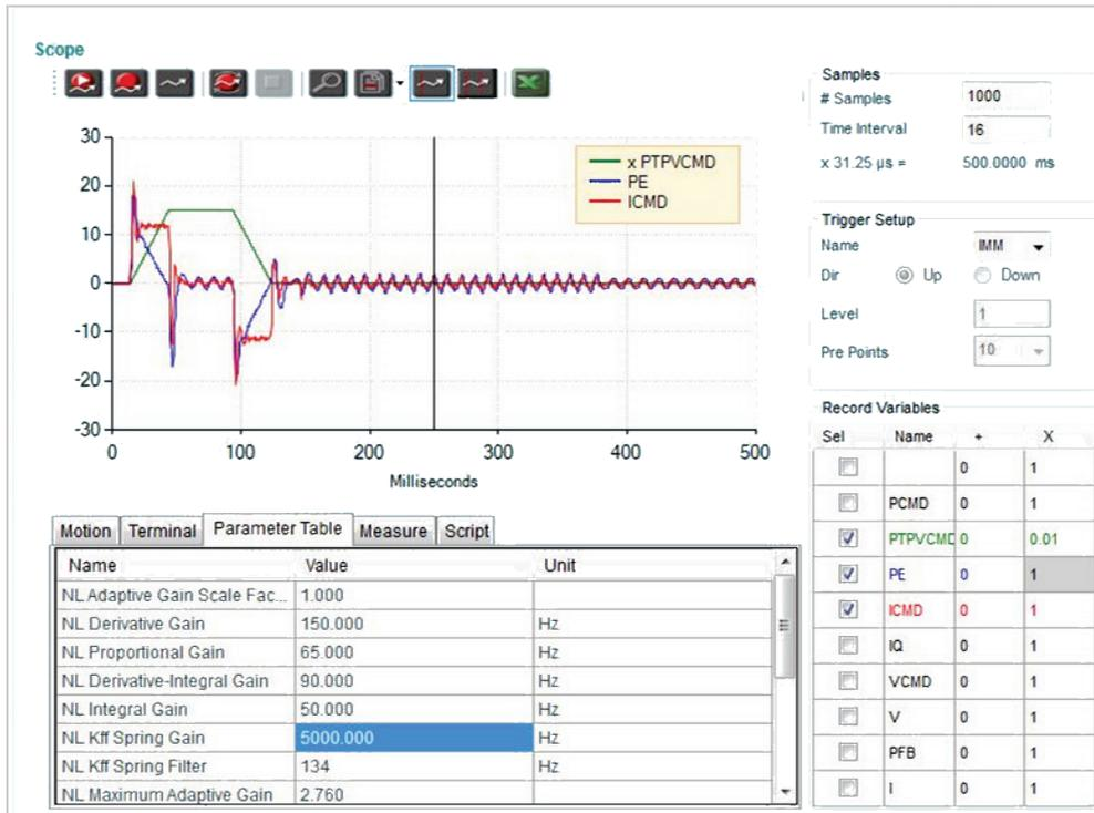
**Figure 12-26.KNLI 50 Hz – Value too high; position error oscillations at stop; overshoot of position error**
