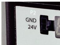
**Figure 3-20. Logic Power 24V Input Interface**
