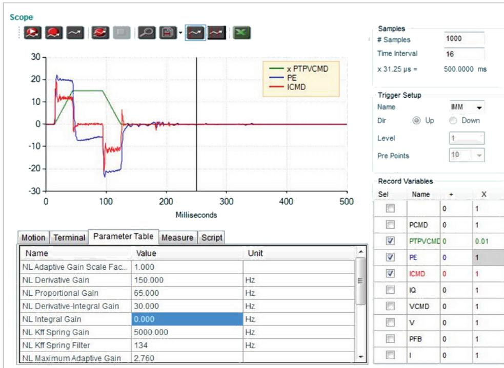
**Figure 12-21.KNLIV 30 Hz - Position error decreases slightly during acceleration and deceleration phases**
