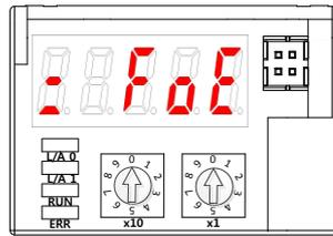
(7-segments display a message when Flash deletion is complete while downloading the firmware using the FoE)
