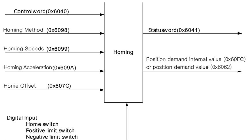
As shown in the figure below, you can set the offset between the home position and the zero position of the machine using the home offset. The zero position indicates a point whose Actual Position Value (0x6064) is zero (0).
