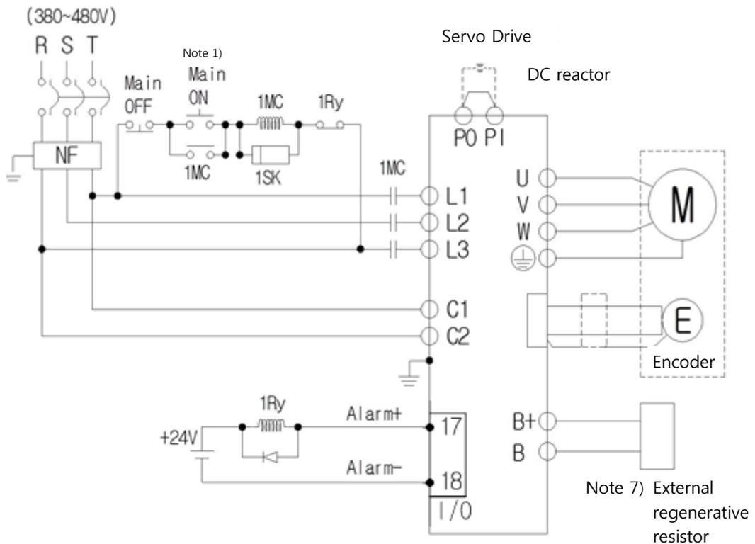
Note 5) It takes approximately one to two seconds until alarm signal is output after you turn on the main power. Accordingly, push and hold the main power ON switch for at least two seconds.
