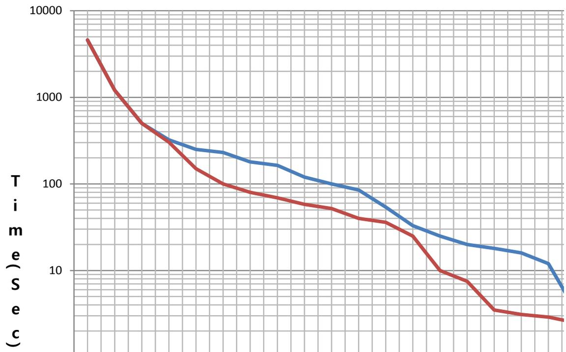
**■ Overload Operating Characteristic Curve (5kW, 7.5kW)**
