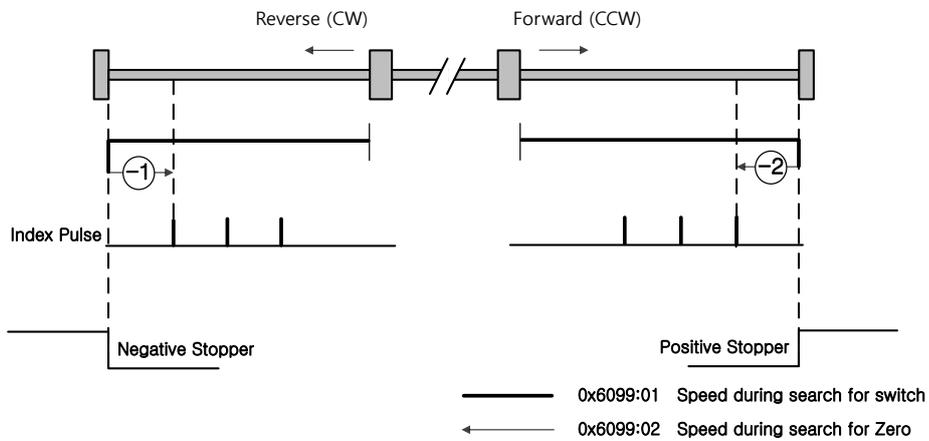
Homing method -1 and -2 perform homing by using the Stopper and Index (Z) Pulse. The velocity profile according to sequence is as follows. For more information, see the details below:
