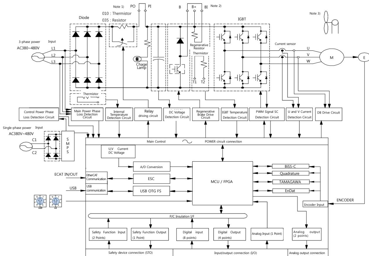
Note 1) If using a DC reactor, connect the PO and PI pins.
