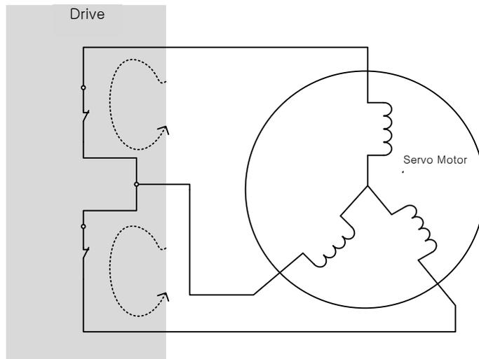
You can set various stop modes, as shown below, in dynamic brake control mode settings [0x2012]:
