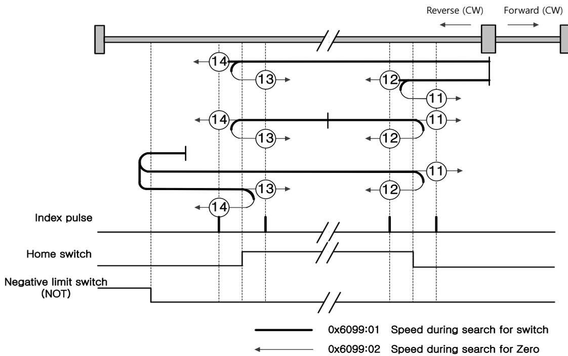
For homing using the Homing Method 14, the velocity profile according to the sequence is as follows. The sequence depends on the relationship between the load position and the Home switch at homing, which is categorized into three cases as below. For more information, see the details below:
