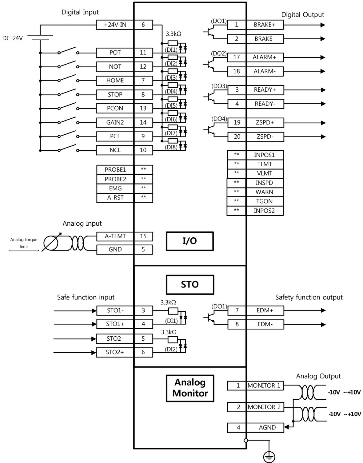
Note 1) The input signals DI1 - DI8 and output signals DO1 - DO4 are the factory default signals.
