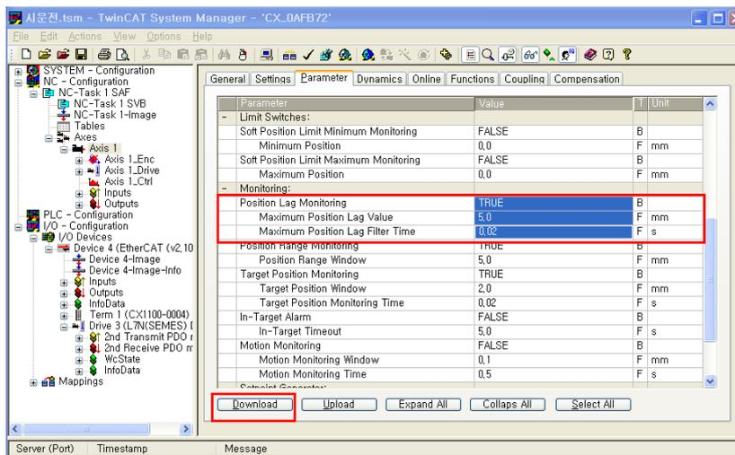
(Note) The Position Lag Monitoring is the difference between the position reference and the actual position at a given cycle time. When the Position Lag Monitoring is enabled, the TwinCAT NC generates an alarm if the positional error exceeds the settings.
