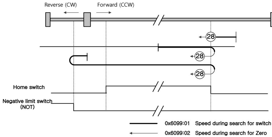
The initial driving direction is reverse (CW), and a point where the Positive Home Switch is turned on becomes the Home position.
