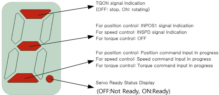
Digit5 indicates the status of the *EtherCAT* State Machine or of the current control mode and servo ON.
