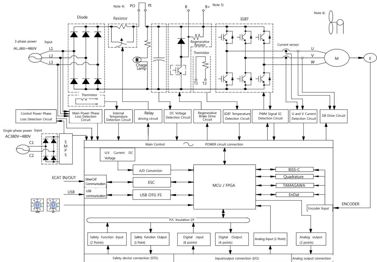
Note 4) If using a DC reactor, connect the PO and PI pins.
