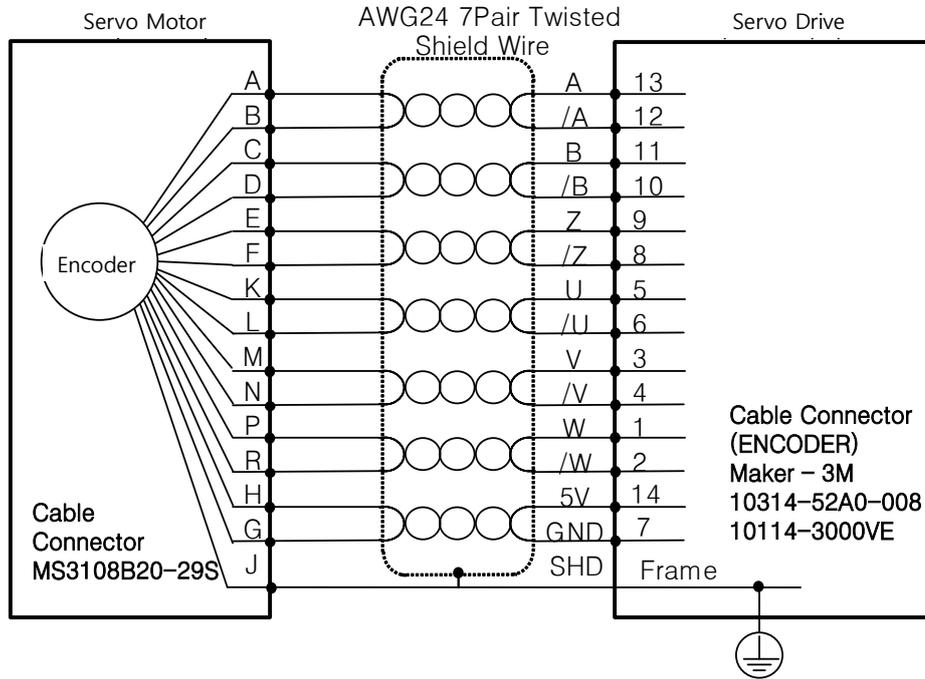
2.6.2 Serial Encoder Signaling Unit Wiring
