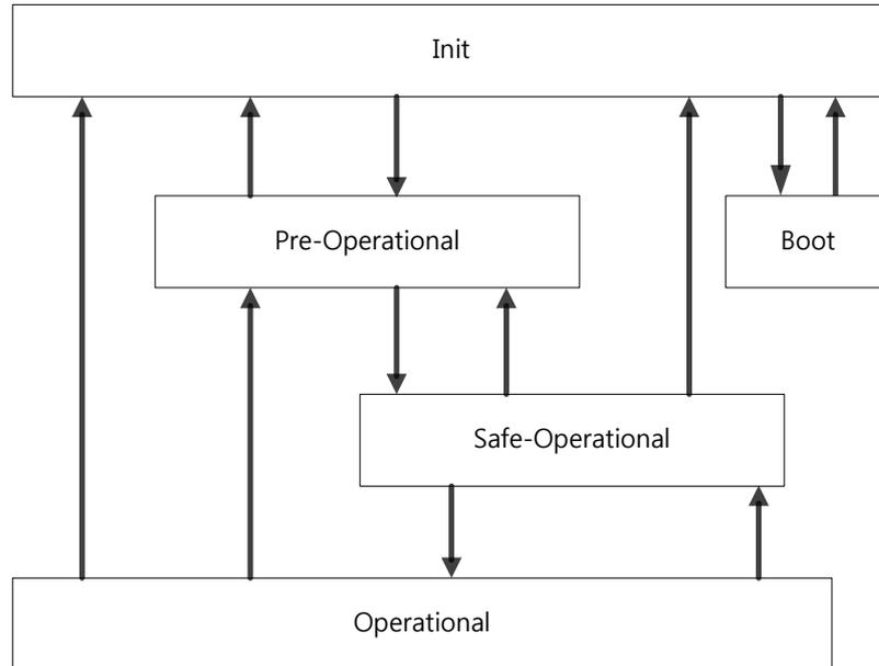
The EtherCAT drive has 5 states as above, and a state transition is done by an upper level controller (master).
