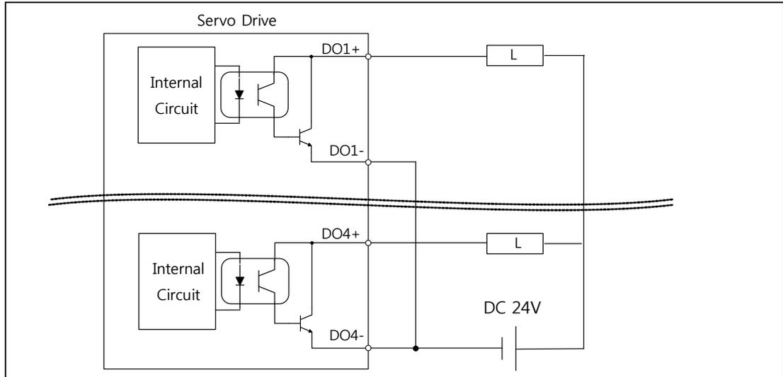
Note 1) For DO1~ DO4 output signals, the GND24 terminal is separated.
