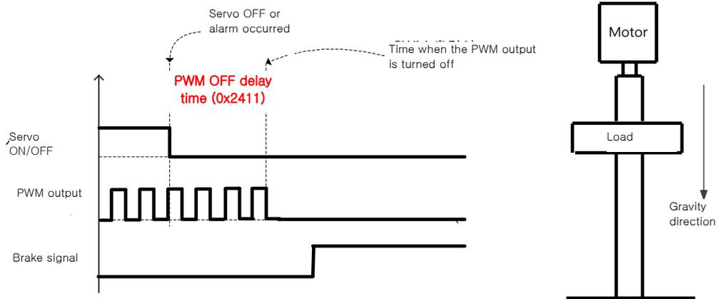
(2) If PWM Output Turns off First Before Brake Signal Outputs
