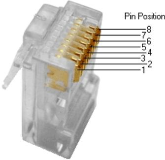
Note 1) EtherCAT only uses signals from No. 1, 2, 3, and 6.
