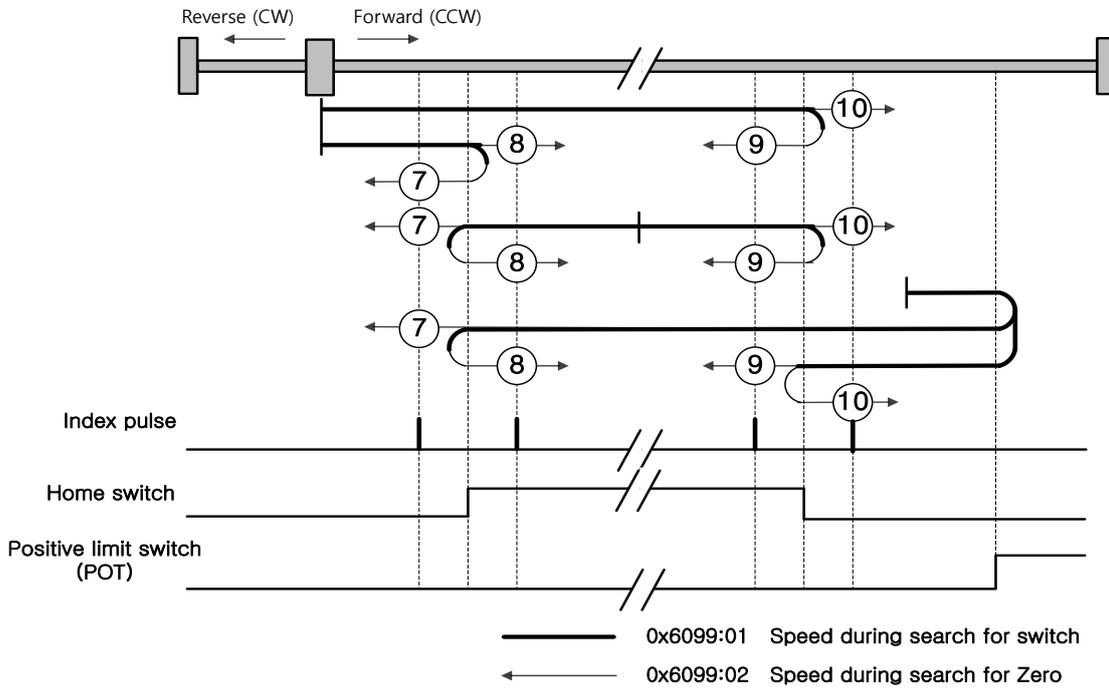
For homing using the Homing Method 7, the velocity profile according to the sequence is as follows. The sequence depends on the relationship between the load position and the Home switch at homing, which is categorized into three cases as below. For more information, see the details below:
