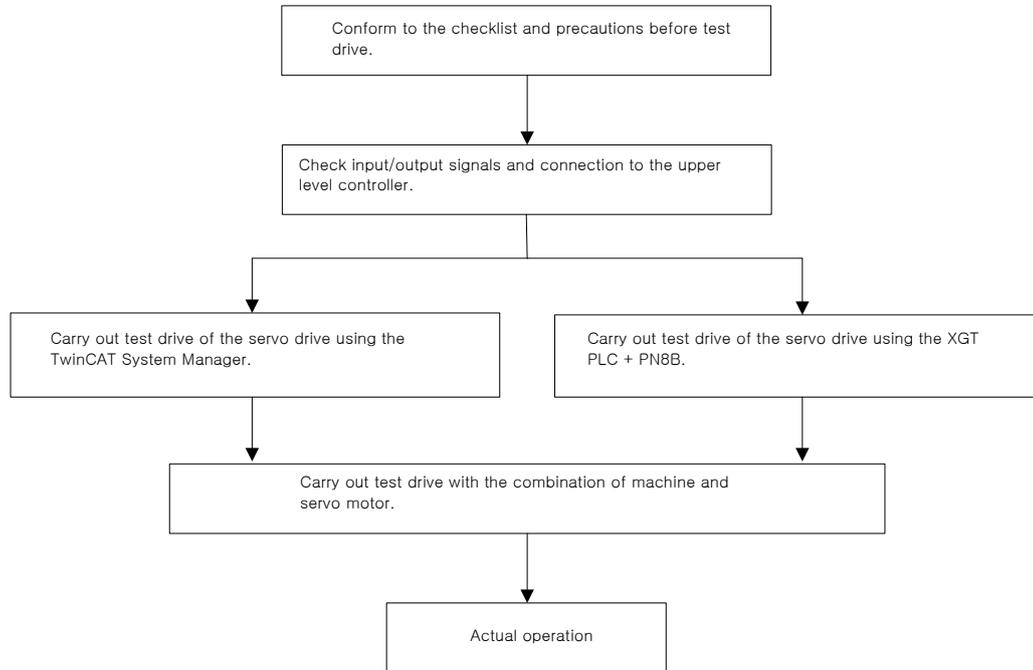
Verify that, before the test drive, the upper level controller and the servo drive are correctly wired, and the objects of the servo drive are correctly configured.
