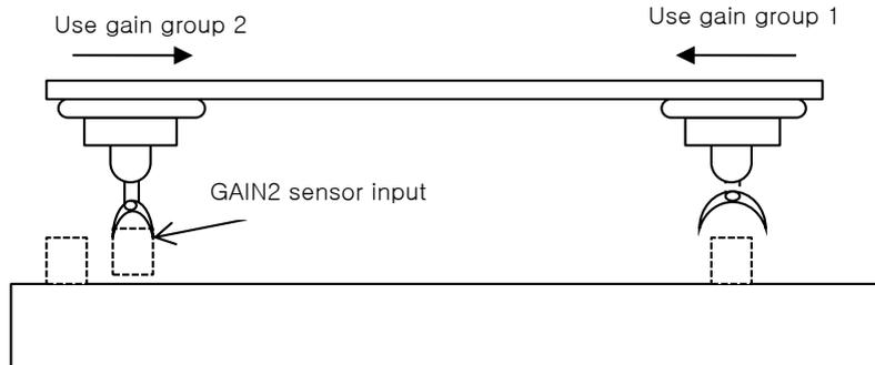
This function is to switch between the gain groups 1 and 2, as one of gain adjustment methods. You can reduce the time required for positioning through switching gains.
