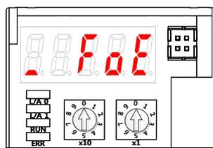
(7-segments display a message when downloading the firmware using the FoE)
