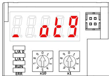
(7-segments display a message when downloading the firmware using the OTG)
