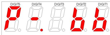
Three digits from Digits 3 to 1 of the 7 -Segment represents the drive status as described below if no servo alarm occurs. In case of servo warning, they will indicate the warning status first, rather than other ones.
