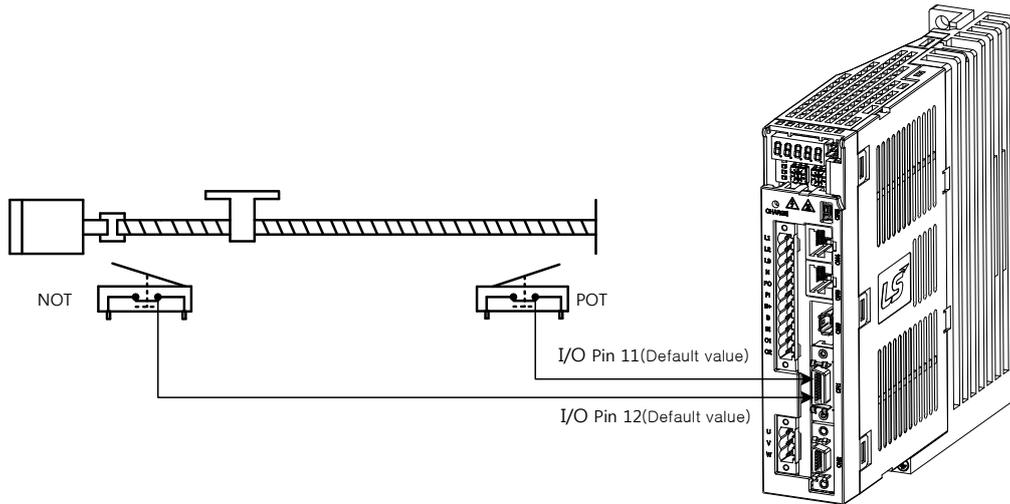
If the positive/negative limit signals are input, the motor will stop according to the emergency stop setting (0x2013).
