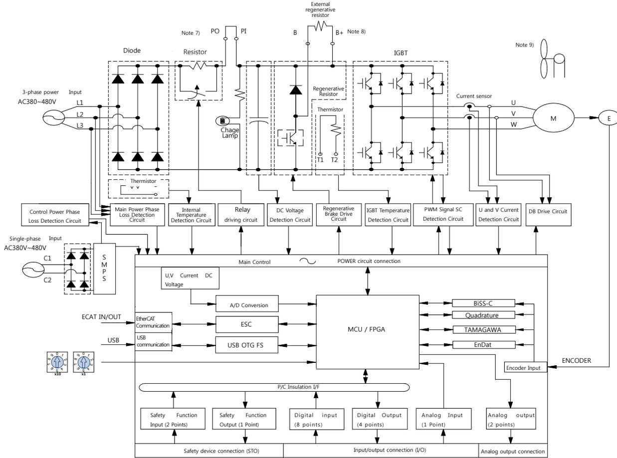
Note 7) If using a DC reactor, connect the PO and PI pins.
