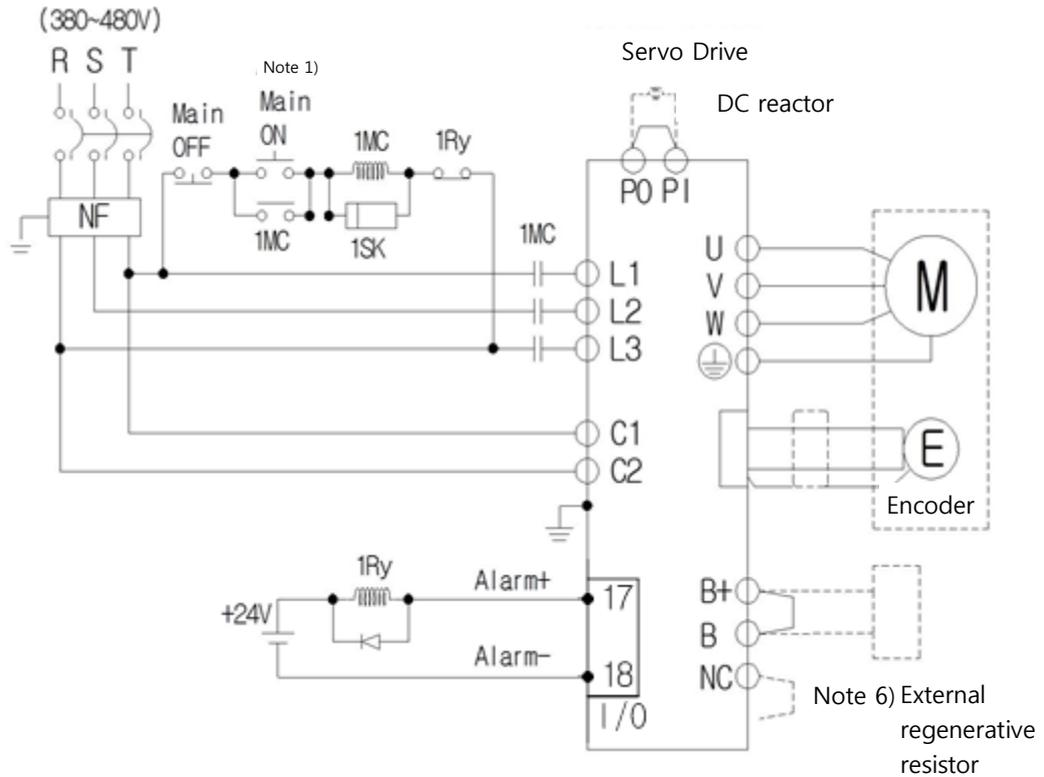
■ Power Supply Wiring Diagram(L7NHB150U)
