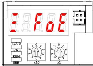
(7-segments display a message when you finished downloading the firmware using the FoE)
