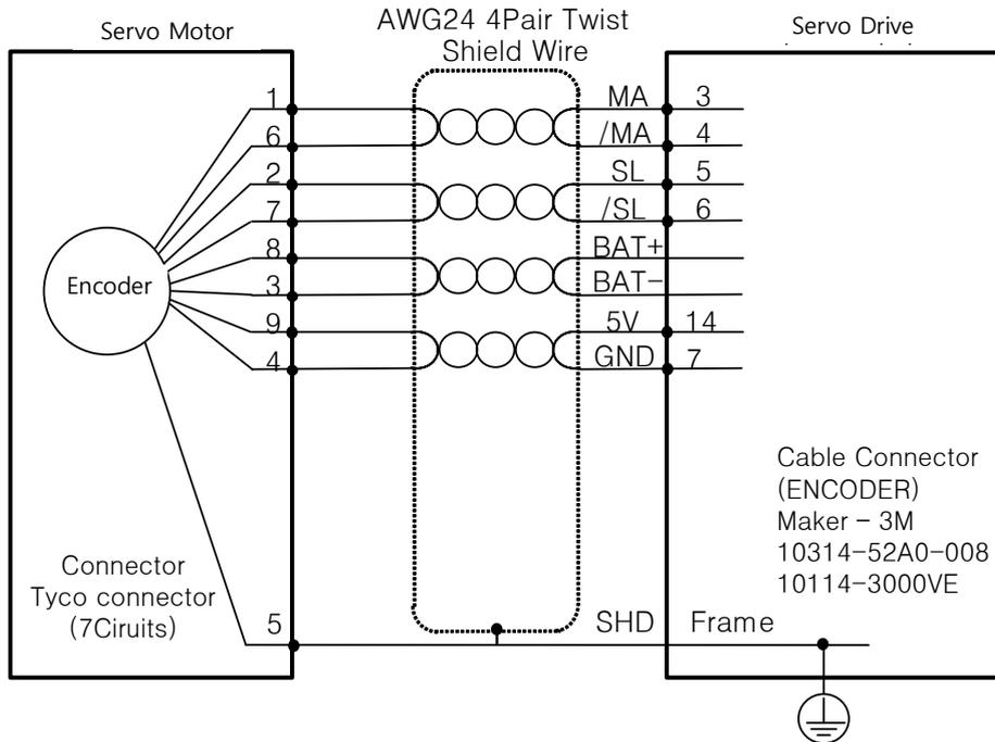
2.6.4 Tamagawa Encoder Signaling Unit Wiring
