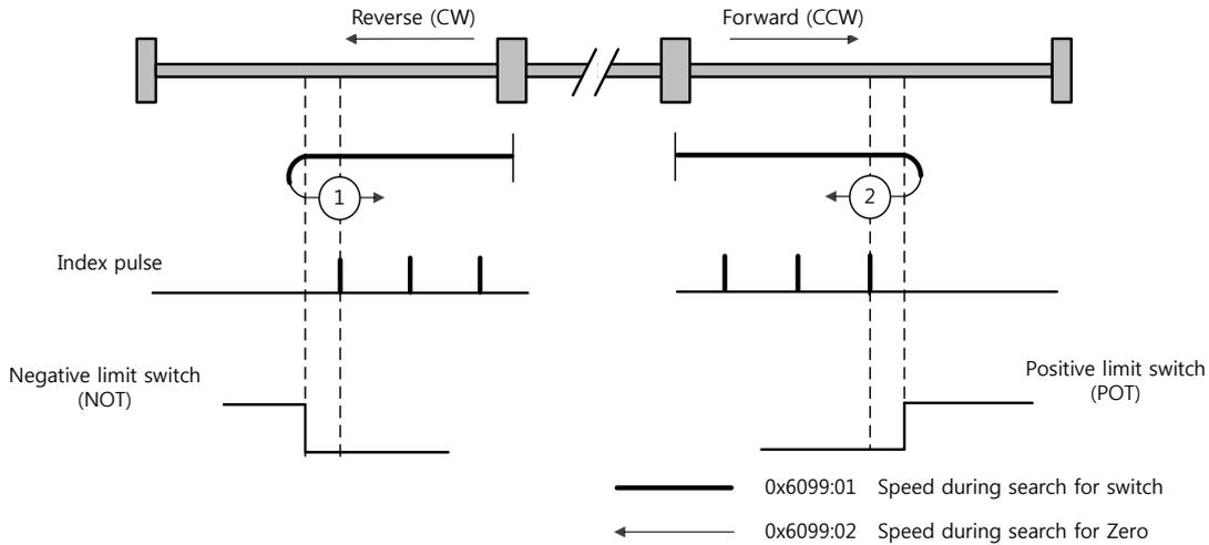
For homing using the Homing Method 1, the velocity profile according to the sequence is as follows. See the details below:
