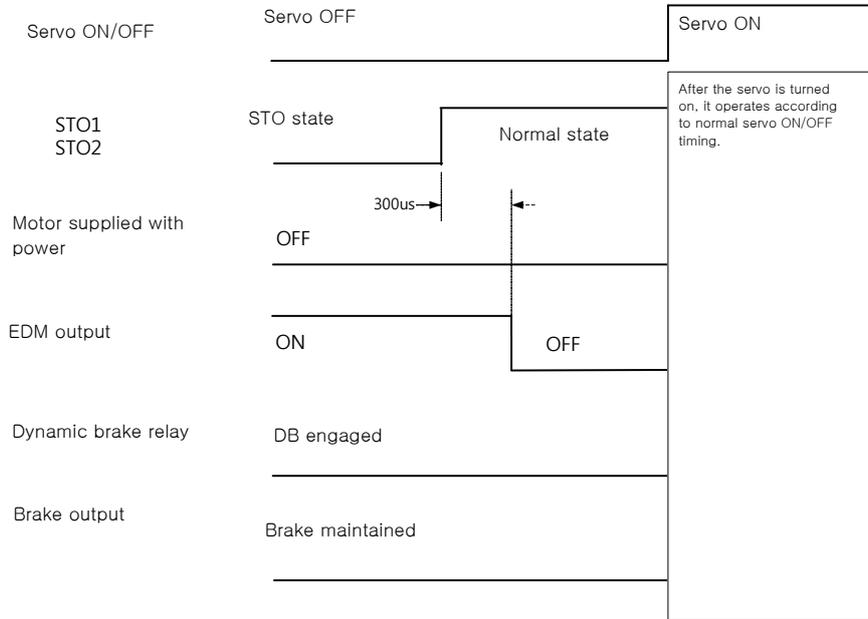
Note 1) Be sure to recover the input signals of STO1 and 2 to ON at the servo OFF state. It is not necessary to reset alarm separately since the "STO state" is not an alarm state.
