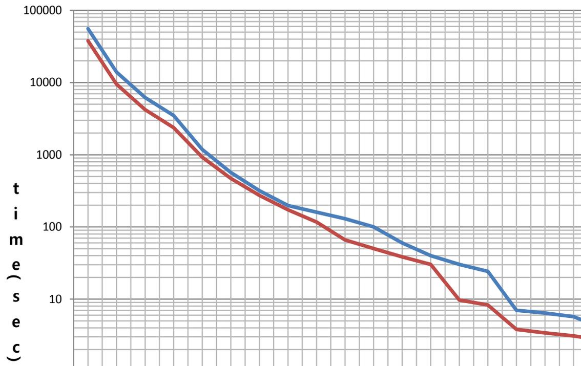
**Overload Operating Characteristic Curve (2kW, 3.5kW)**
