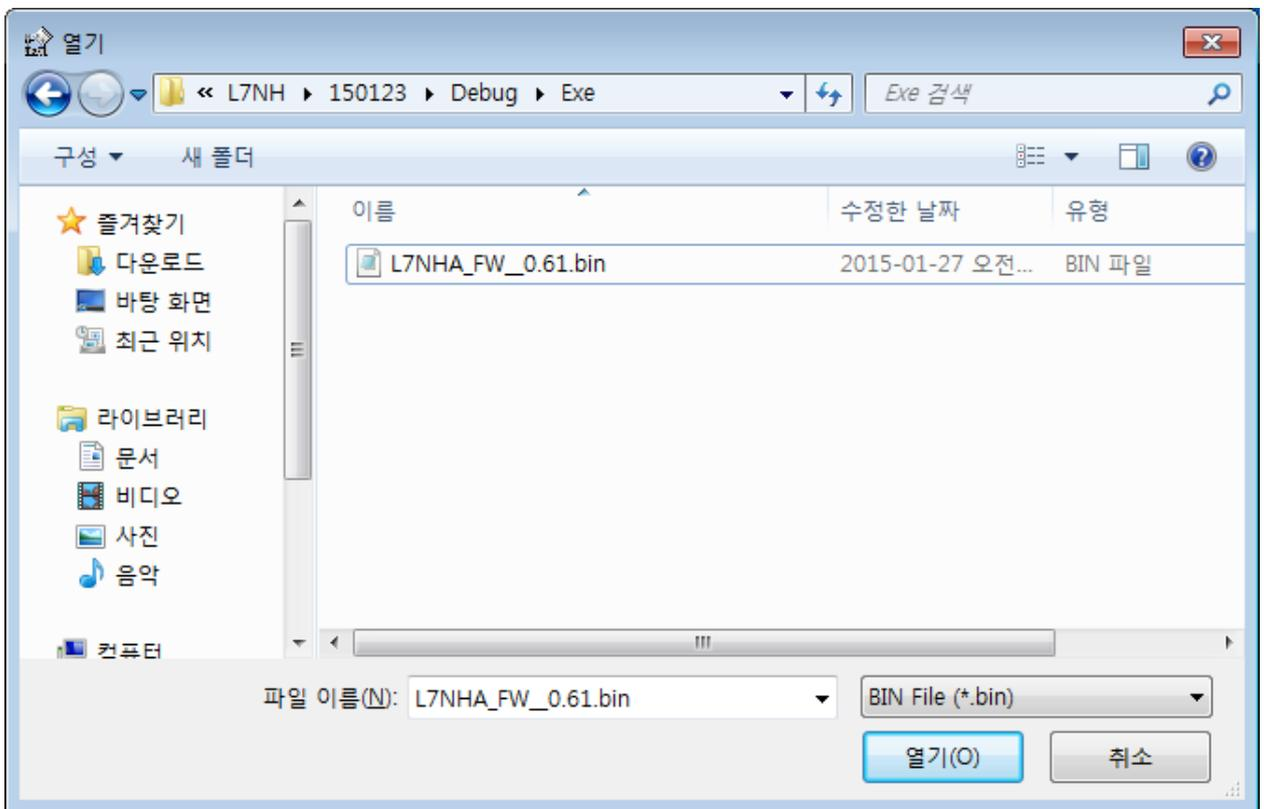
3) Select the BIN file of the firmware to transmit and press the Open button.
