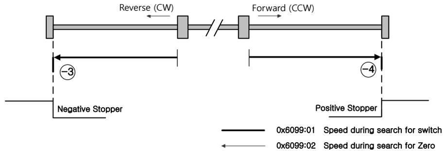
Homing method -3 and -4 only perform homing by using the Stopper. The velocity profile according to sequence is as follows. For more information, see the details below:
