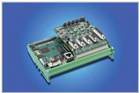
Figure A2.1: AMP-20440 mounted on DMC-2145-DIN
