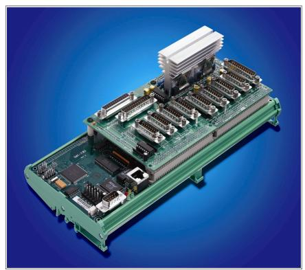
Figure A1.1: ICM-20100 (left) and AMP-20341 (right) mounted on DMC-2185-DIN
