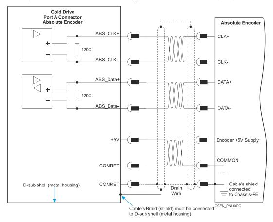
Figure 23: Absolute Serial Encoder - D-Type Connection Diagram Example
