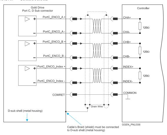
Figure 36: Encoder Differential Output – D-Type Connection Diagram Example
