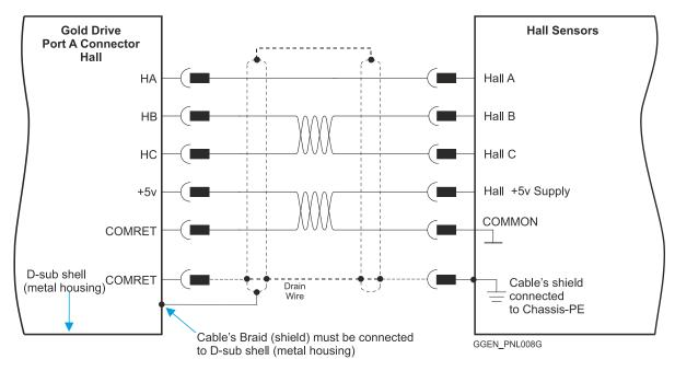
Figure 21: Hall Sensors D-Type Connection Diagram Example
