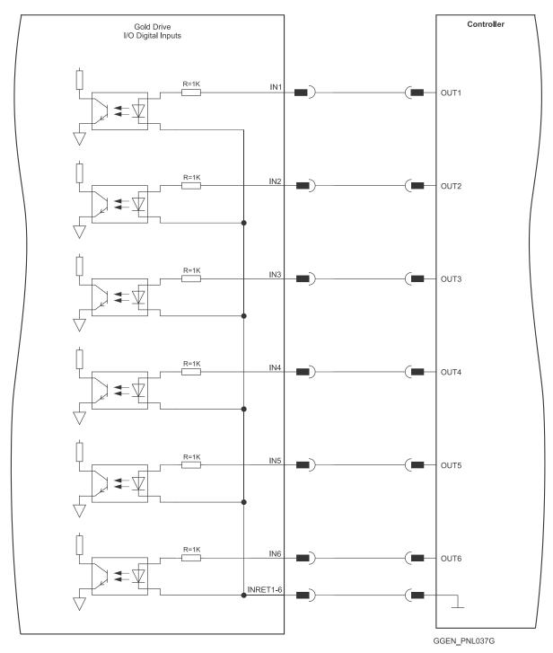
Figure 44: Digital Input TTL Mode Connection Diagram Example
