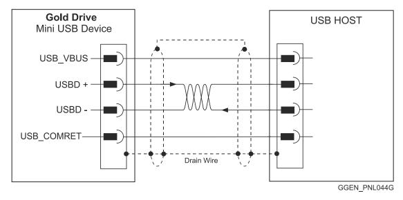
Figure 57: USB Network Diagram Example
