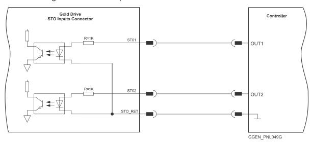
Figure 11: STO Input Connection – TTL Option
