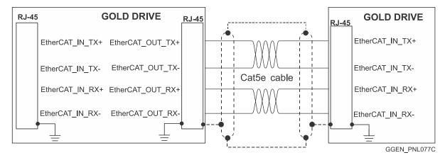
Figure 58: EtherCAT RJ-45 Connections Example
