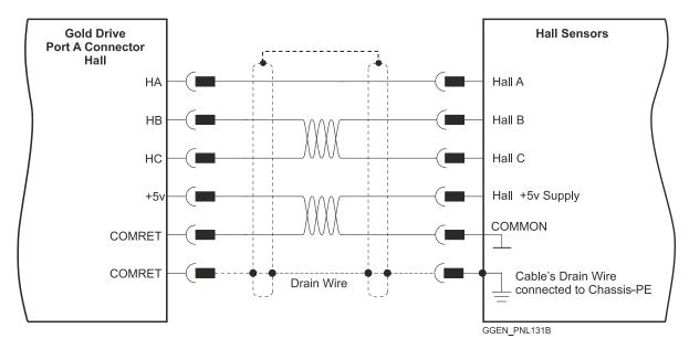
Figure 22: Hall Sensors Shrouded Type Connection Diagram Example
