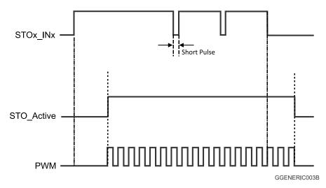
Figure 7: Timing Diagram of short pulses
