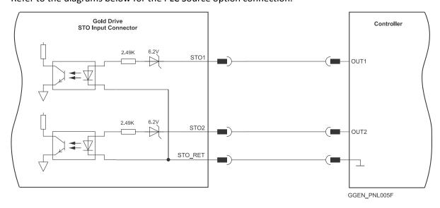
Figure 9: STO Input Connection Example – PLC Source Option
