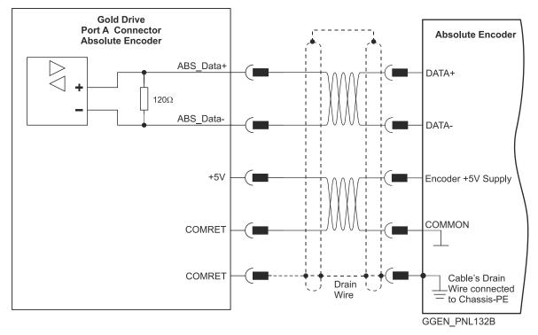
Figure 26: Absolute Serial Encoder – Shrouded Type Connection Diagram Example for Sensors Supporting Data Line Only (NRZ types, e.g., Panasonic / Tamagawa / Sanyo / Nikon)
