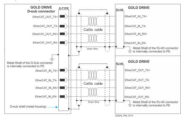
Figure 60: EtherCAT with D-TYPE Connections Example
