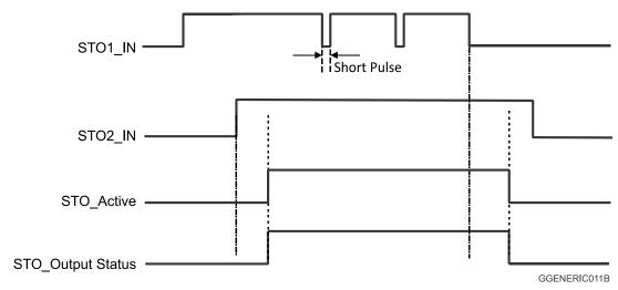
Figure 13: STO Output Status Timing Diagram (Refer to STO Timing)
