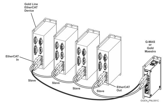
Figure 63: EtherCAT Network with Redundancy
