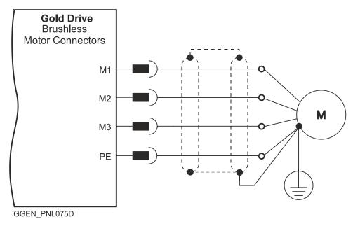
**Figure 3: Brushless Motor Power Connection Diagram**
