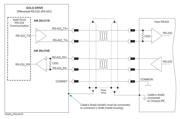
Figure 67: Differential RS-232 D-Type Communication Example
