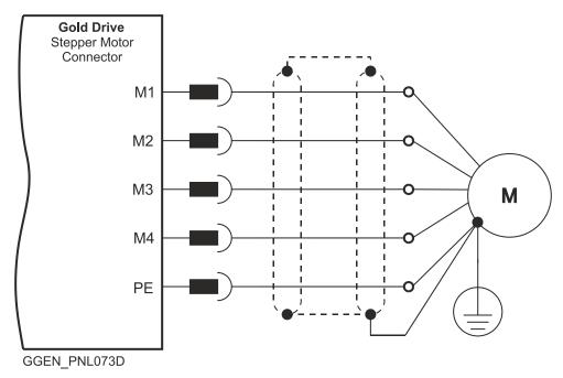
**Figure 5: Stepper Motor Power Connection Diagram**
