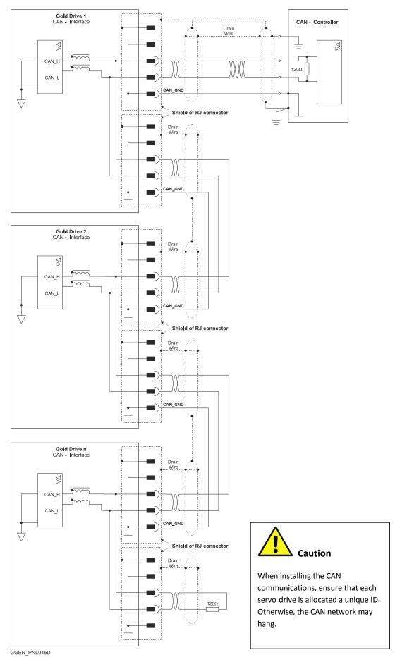
Figure 64: Gold Panel Mounted Servo Drive Connection Diagram Example – CAN
