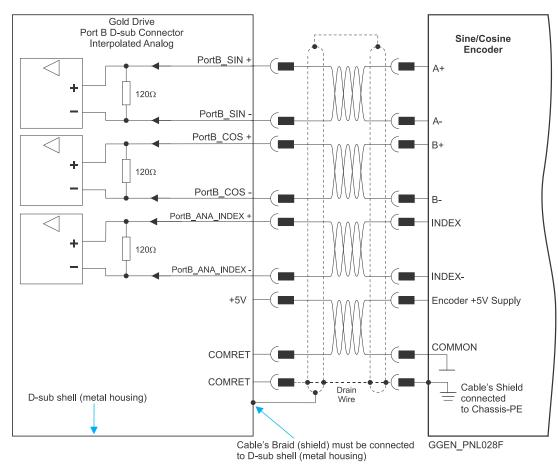
Figure 32: Port B - Interpolated Analog Encoder D-Type Connection Diagram Example
