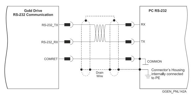
Figure 66: RS-232 RJ-45 Connection Diagram Example
