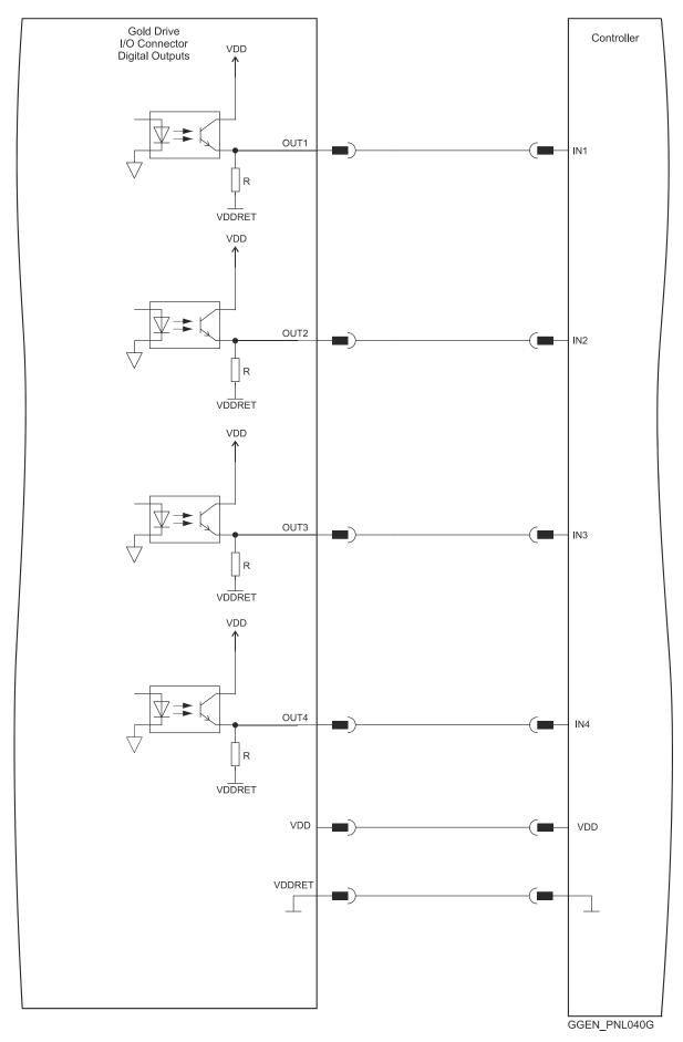
Figure 46: Digital Output Connection Diagram Example – TTL Option
