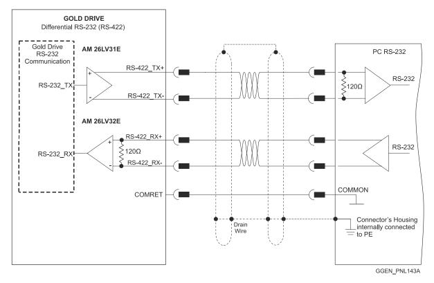
Figure 68: Differential RS-232 RJ-45 Communication Example
