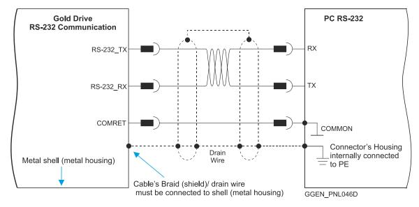
Figure 65: RS-232 D-Type Connection Diagram Example
