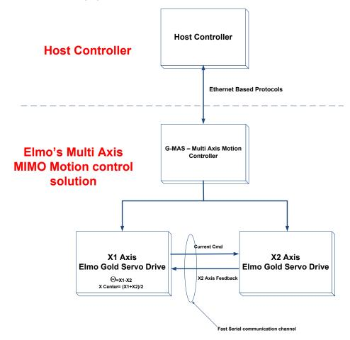
Figure 38: Flexible Gantry system
