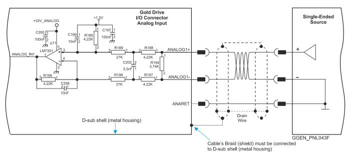
Figure 55: Differential Analog Input for D-Type connector
