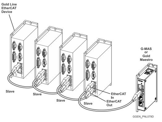
Figure 62: EtherCAT Network with No Redundancy
