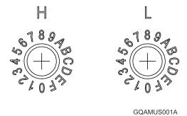
Figure 61: EtherCAT Address Switches
