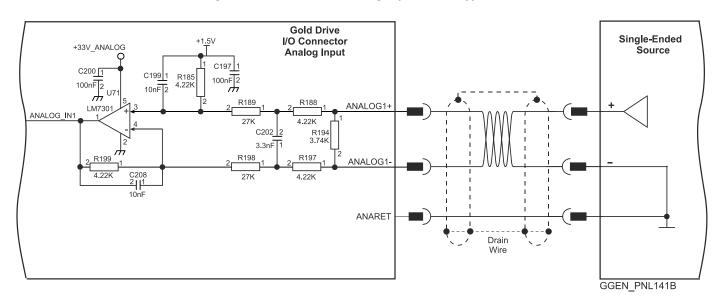
Figure 56: Differential Analog Input for Shrouded Type connector
