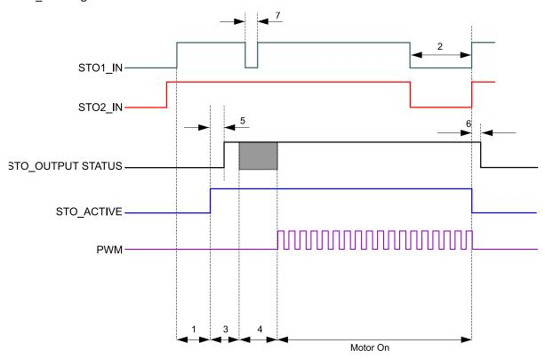
Figure 15: STO Timing Diagram
