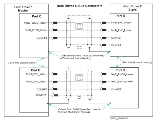
Figure 41: Port C to Port B D-Type Connections
