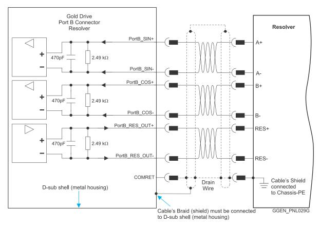
Figure 34: Port B – Resolver D-Type Connection Diagram Example
