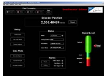
SmartPrecision™ Software The software module enables all programmable and diagnostic features plus displays encoder output and signal strength. See page 8 for details.
