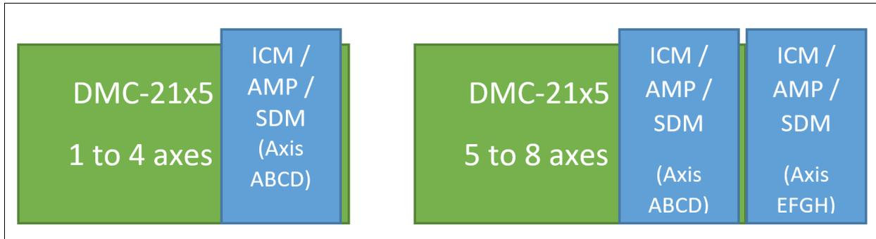
Figure 1.1: Layout of DMC-21x5 with one bank of axes and layout of DMC-21x5 with two banks of axes
